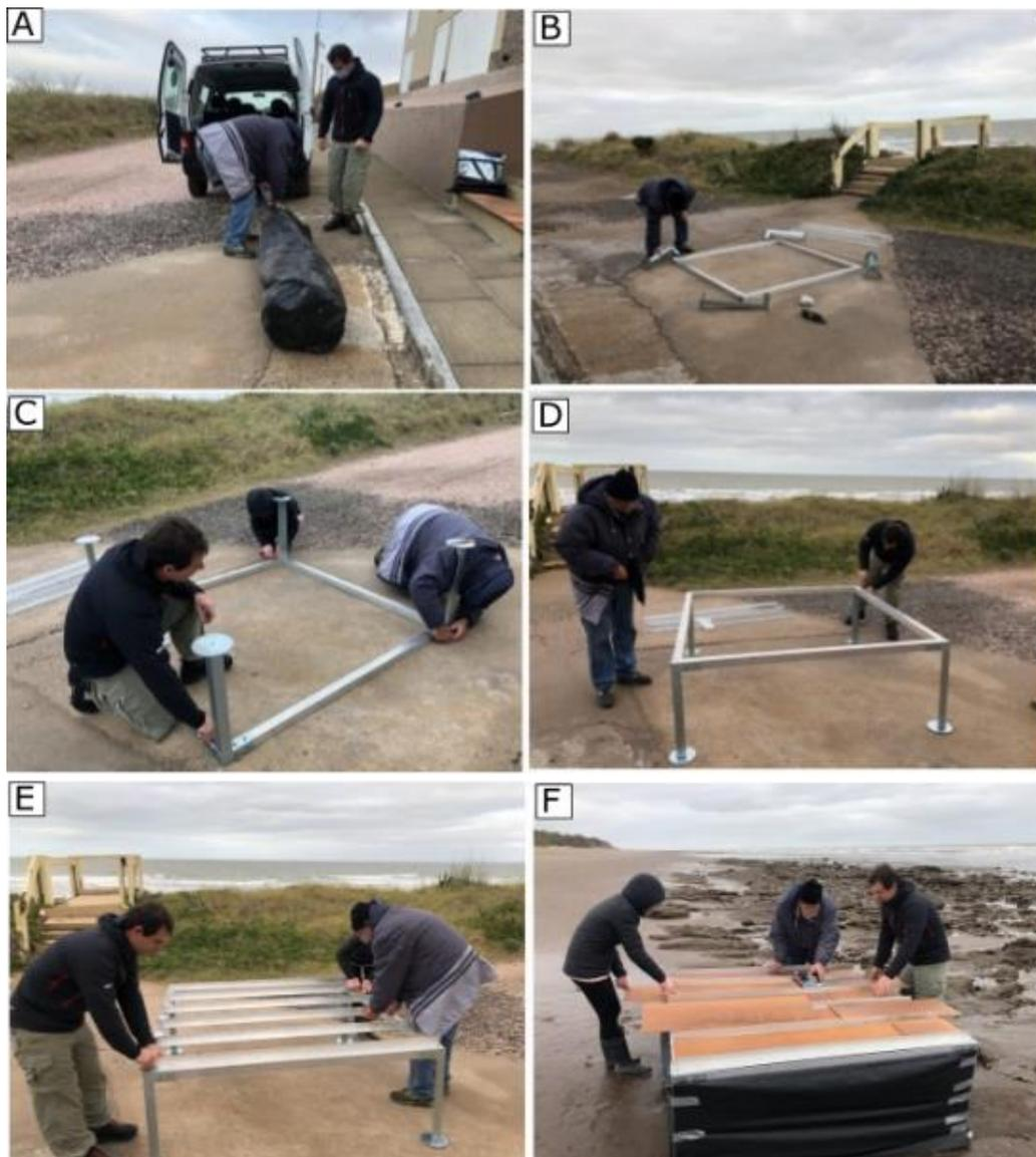
**Figure 2.** MiSMoS assembly stages. **a)** Storage of MiSMoS pieces, **b)** pre-assembly inspection of the structure, **c)** addition of supports and screws, and **d)** placement of supports for curtains. **e)** Incorporation and adjustment of aluminum rails to the MiSMoS structure frame, and **f)** movement of the sensor-carrying and panels that block light during the survey.
