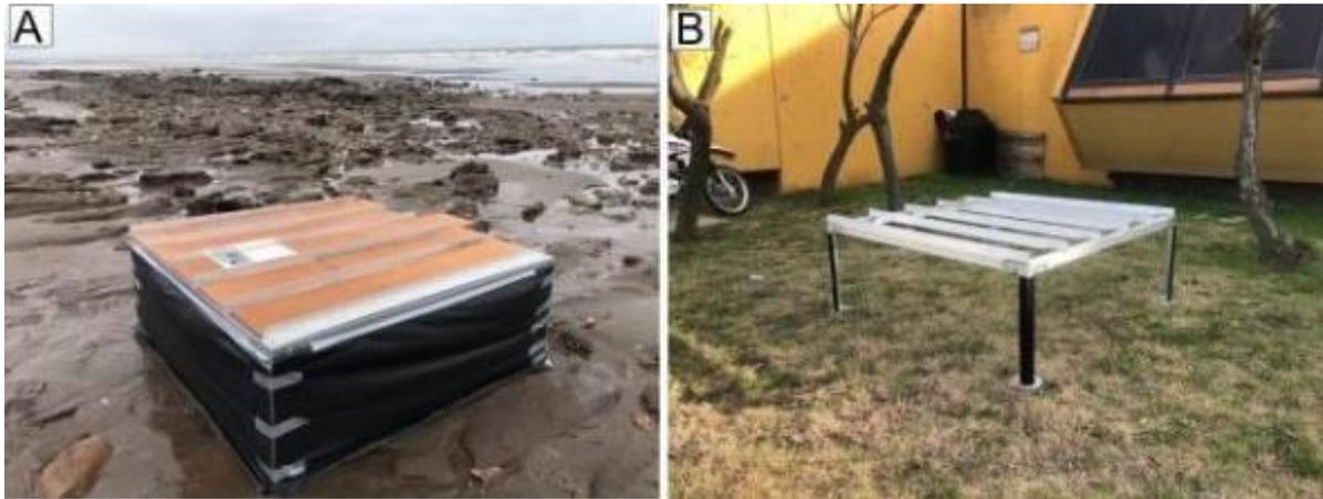
**Figure 3.** External light control. **a)** side section covered curtains and the black faux leather fabrics secured to the structure supports with tape, and **b)** supports velcro straps on the sides.
